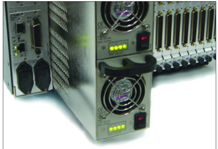
Hot-swap power supplies Most products feature hot-swap monitored supplies
