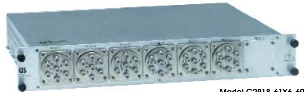
Model G2R18-61X6-60 Six sections of 1x6 DC-18GHz relays with SMA connectors
