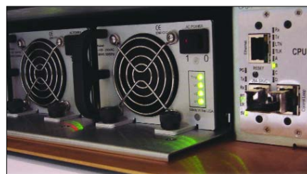
Front mounted hot-swap power supplies
