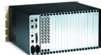
Model S2084E Rear-facing twenty-position vertical module bay and dual CPU bay
