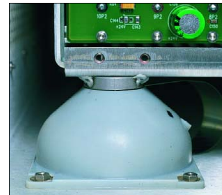
Special shock mounting Our ruggedized VXI chassis features internal shocks
