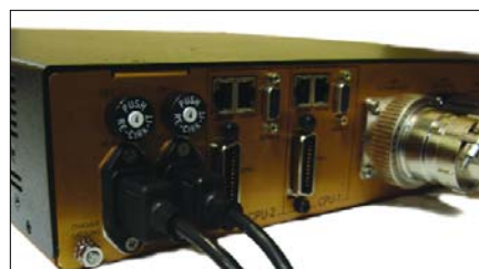
Dual AC inputs and redundant control ports
