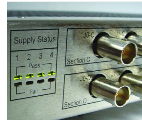
Monitored power supplies Power supplies are monitored for proper operation
