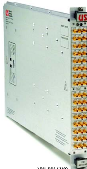
VXI-RR161X2 Sixteen 1x2 relay sections DC-1.3GHz with SMB connectors
