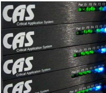
Liberal use of status indicators Indicators help during system set up and troubleshooting
