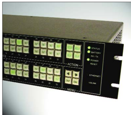
LED control keys All units contain LED backlighting, no bulbs
