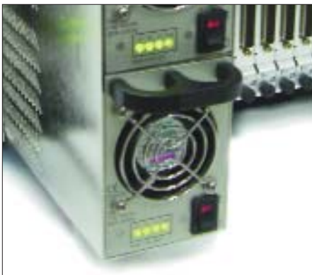
Hot-Swap power supplies Most products feature hot-swap monitored supplies
