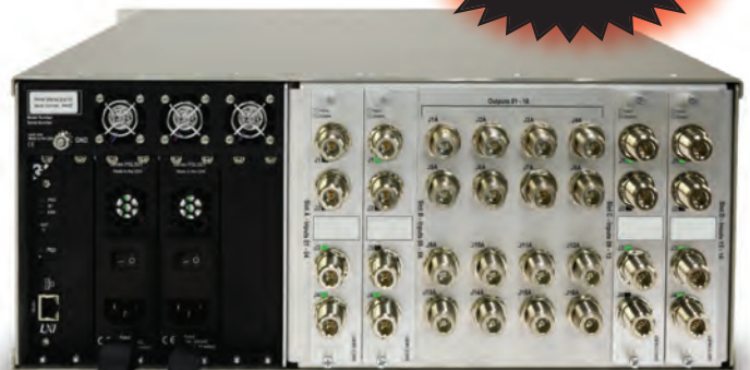
SWM16X N-Type connectors Optional dual CPU Optional LNB power & control, gain, AGC
