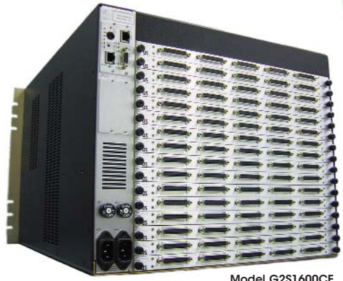
Model G2S1600CE Sixteen-slot G2 Mainframe Rear view with modules installed (8RU)
