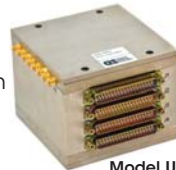
Model U6048-50 Compact reed relay blocking matrix (DC-100MHz)
