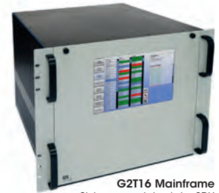
G2T16 Mainframe Sixteen module slots, 8RU (shown with Option X display)
