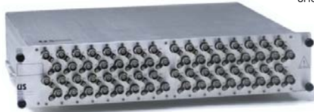
G2S47-6432-25 G2 plug-in 32x32 IF matrix with expanders (20-250MHz) Page 8 & 9
