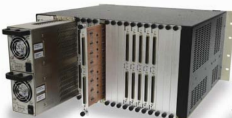
New S64530 RS-530 Digital Router 64X64 with Adapter Panels
