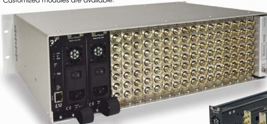
Updated LS16A showing the "Open Window" front panel design w/test points & LEDs
