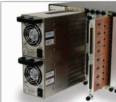
Hot-Swap power supplies & modules Most products feature hot-swap monitored supplies, control CPUs, and modules
