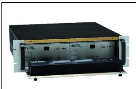
Front view with hinged front panel open exposing dual (redundant) plug-in power supplies.
