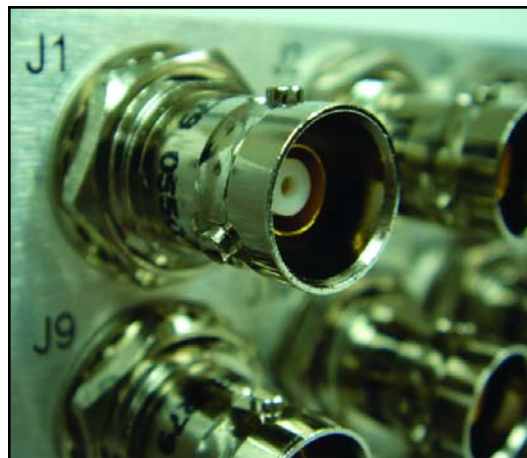
Close up of the 3-Lug Triax connector, (sometimes referred to as a "concentric twinax" connector)
