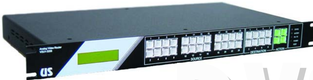
Model DVSU1-3208 24 input, 8 output
