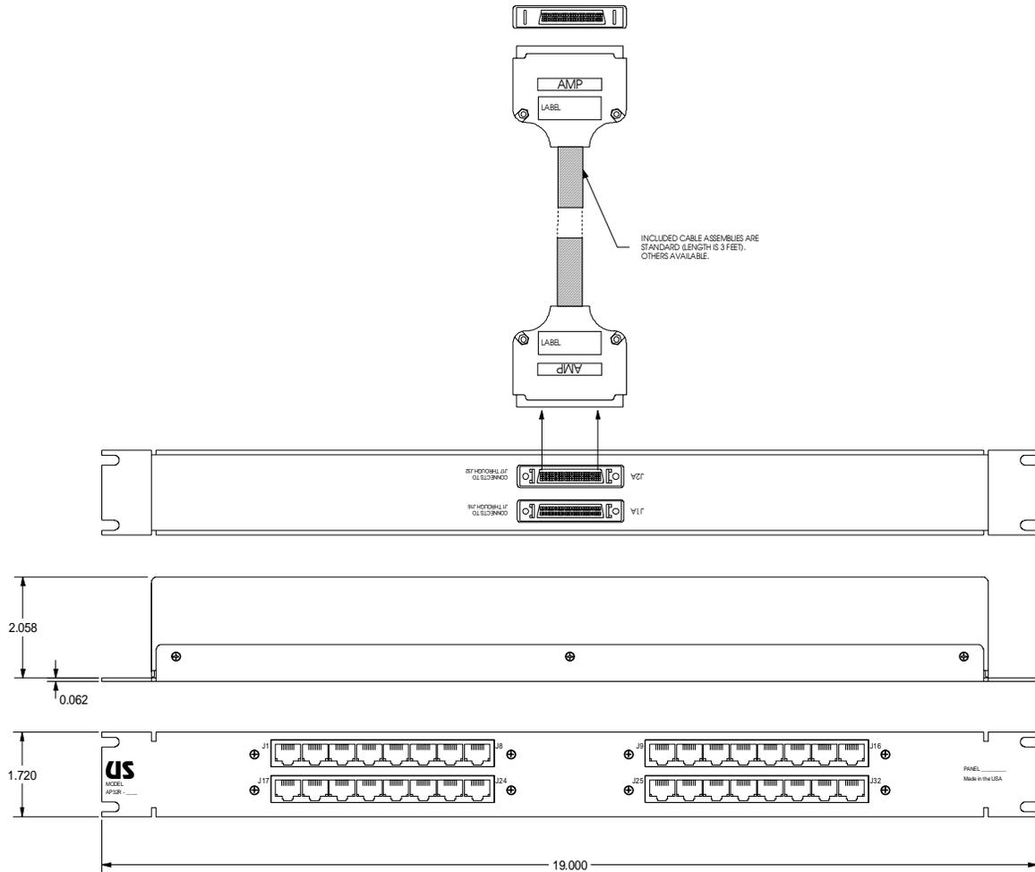
It is designed to route both input connectors on an input module on the S2560D, both output connectors from an S2560D module, or one of each (half input and half output). Below is an S2560D unit with sixteen AP32R units attached for a total configuration of 256 inputs and 256 outputs and RJ45 connectors.
