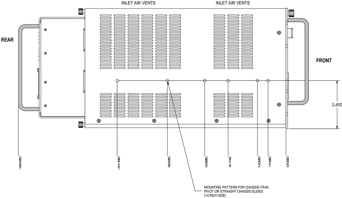
The unit is designed to install in a standard 19" equipment rack. It is comprised of an individual rack mountable mainframe with plug-in modules. All user signal I/O and control signal connections to the unit are at the rear, and therefore would come from inside the equipment rack enclosure.
