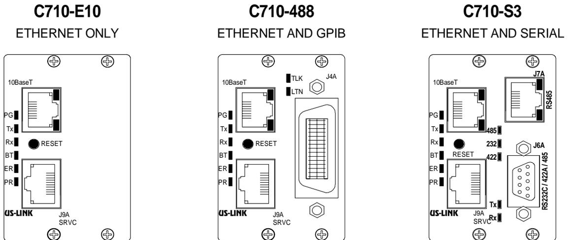
The unit model number determines the type of CPU that is included when the unit is delivered from the factory. Some unit configurations can have two of these assemblies installed for additional flexibility or for a redundant means of control. These CPU assemblies install into the rear of most systems and are secured by two phillips-head screws at the top, and two at the bottom.
