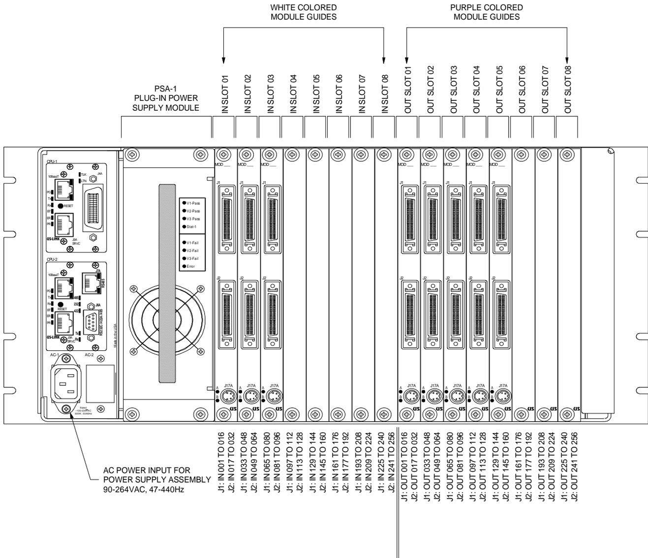
The unit can be expanded by adding additional modules while it is in the field. The unit's firmware automatically senses the newly installed modules and responds accordingly. All I/O modules plug into the rear of the unit, are hot swappable and are secured to the chassis by two captive fasteners.
