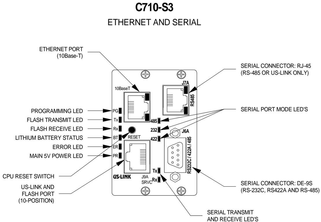
The plug-in assembly is part of the Series C710 interface/CPU product line. The complete model number is C710-S3 and includes the following features
