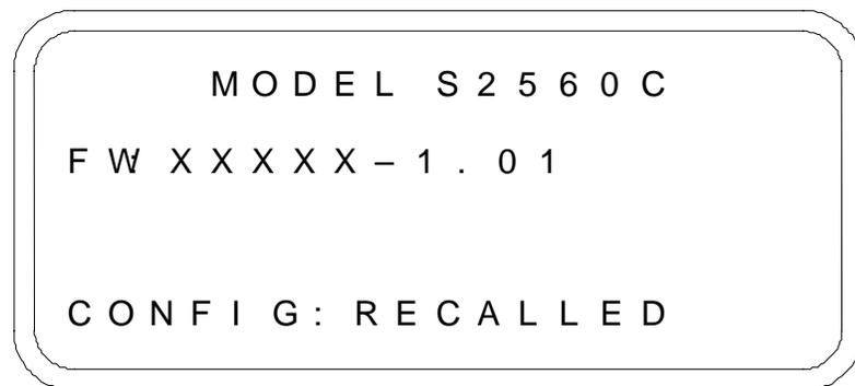
The bottom line of this screen indicates if the unit is recalling the last configuration prior to power-down, or if the configuration is "cleared" of all crosspoint configuration closures. This is a menu selection at the front panel for AUTO RESTORE (yes or no).
