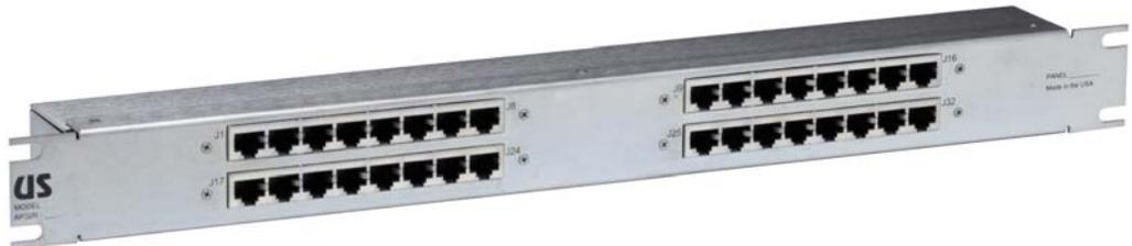
The AP32R is a totally passive and bi-directional unit that can be connected to the System S2560D. It provides the user with up to 32 individual RJ45 connectors, each providing a single pair of signal paths. It can be used for either input or output signal routing.
