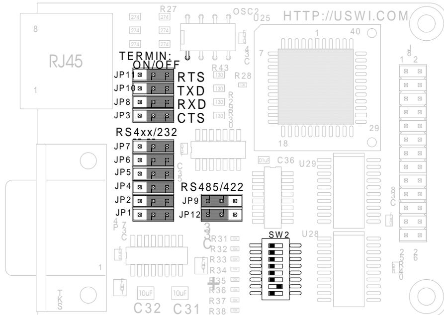
The jumpers are moved to different positions to properly connect drivers and receivers for the different serial modes. The diagram below shows how the jumpers and dipswitch are to be positioned for the different formats.
