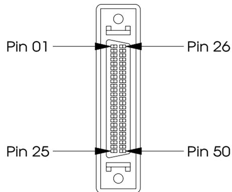
The connector is an AMP #749649-5 and is part of the SCSI-II family of connectors. Different configurations of mating connectors could be used, one being AMP #749110-1. This is just the mating portion of the connector and does not include a back-shell.
