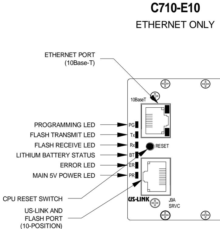
The plug-in assembly is part of the Series C710 interface/CPU product line. The complete model number is C710-E10 and includes the following features:
