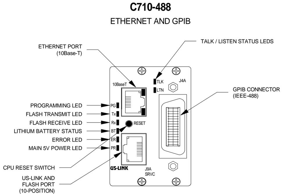
The plug-in assembly is part of the Series C710 interface/CPU product line. The complete model number is C710-488 and includes the following features:
